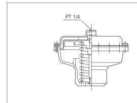
This type is exclusively used for rotary valves. The nose of the diaphragm is free, and by attaching a link, linear motion of the actuator is smoothly converted to rotational motion of the valve stem. Diaphragm features friction-free operation, excellent efficiency, and high output.
